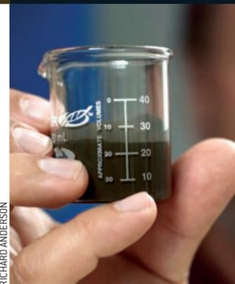
Silver nanoparticles are suspended in an emulsion of water and oil in Cima Nano-Tech's Self Aligning Nano Technology for Electronics, or SANTE™ process.
